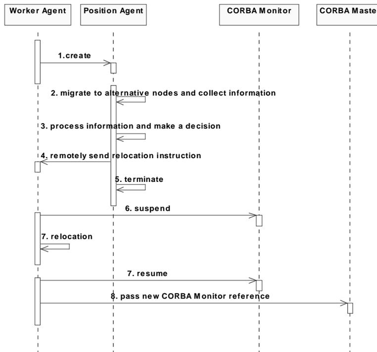
**Fig. 4.** A typical relocation scenario
