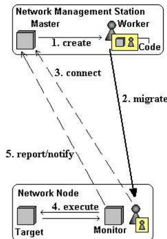
**Fig. 3.** Initiation of the performance monitoring task
