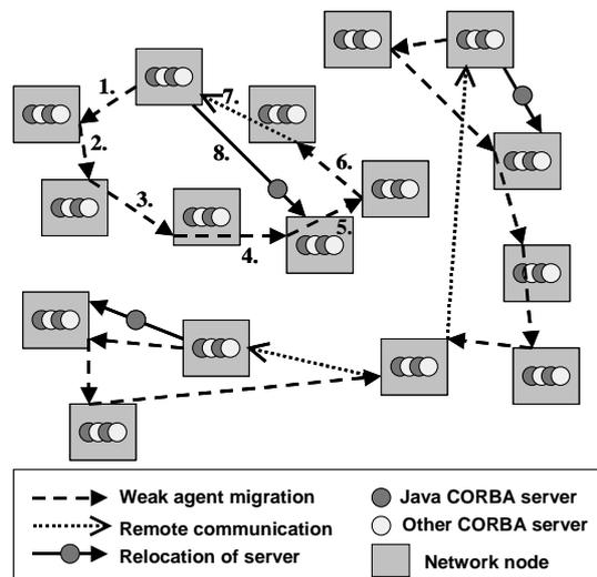
**Fig. 1.** A system of dynamically positioned Java-based CORBA servers
