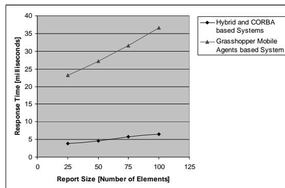
**Fig. 5.** Response times for the transmission of performance reports
