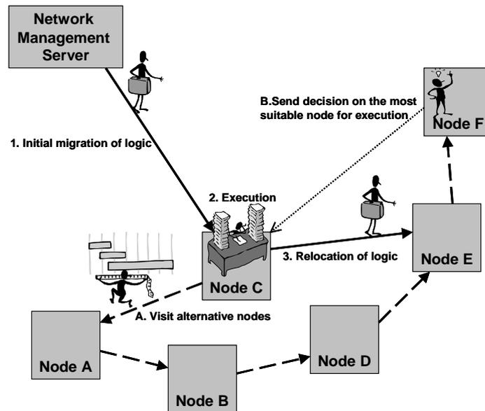
**Fig. 2.** A typical scenario of operation and re-location of a single Java-based CORBA server
