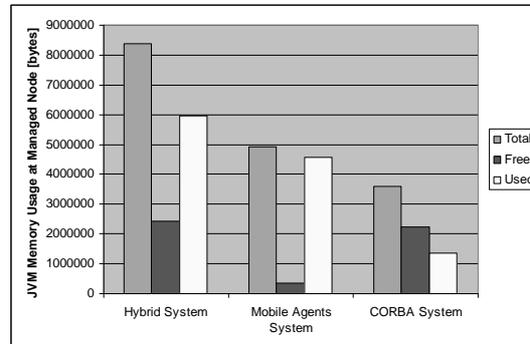
Fig. 7. JVM memory usage at a managed node
